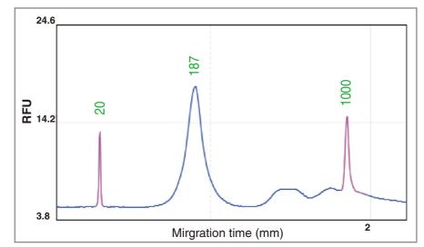
cfDNA were purified by iCATCHER from 4ml plasma sample then ran capillary electrophoresis on BiOptic Qsep 1. iCATCHER can catch clear and sharp peak of cfDNA.
